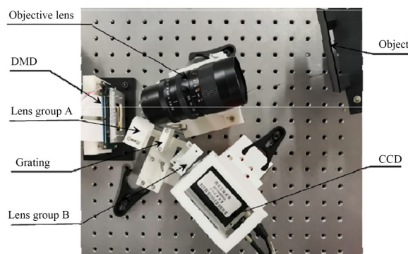
(b) 基于DMD的高光谱成像系统 [65] (b) Hyperspectral imaging system based on DMD [65]
